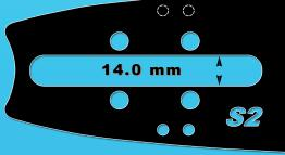
S2 mount fits chainsaws equipped with 14.0 mm bar studs. ie. - Stihl 084, 088 & 090. Dolmar 122, 123, 143, 144, 152, 153 & 166. Olympyk 999.
